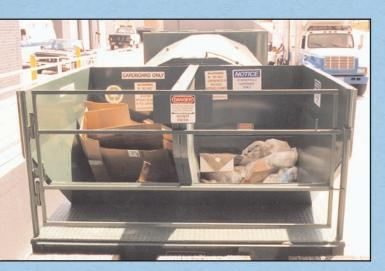
At this large hospital, the DRC II averages 60% trash in one compartment and 40% cardboard in the other compartment. This provides convenience and flexibility while requiring only one unit.
