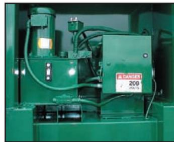
The side mounted power unit offers easy access for maintenance on the motor and electrical panel.
