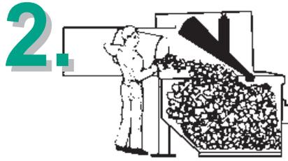
2. The large door opening allows even a 30 gallon container to be emptied easily. The new waste material is dumped into the cavity left in the container by previous ram position.
