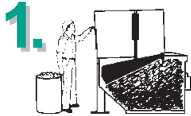
1. Operator inserts key and turns to "UP" position. When ram moves up position the door can be opened.
