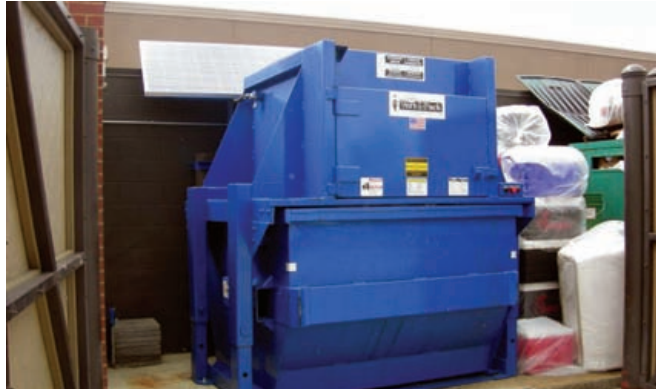
This VIP, located at a national fast food restaurant, features the GreenBuilt® Solar Powered Power Unit Option. The solar panels provide up to 100% of the power requirements. The solar energy is directed into 2 premium deep cycle batteries.
